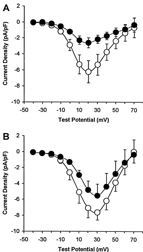
Fig. 3. Mean whole-cell  $\text{Ca}^{2+}$  channel current-voltage relationships (with vertical SEM bars) recorded in the absence (open symbols) and presence (filled symbols) of 2  $\mu\text{M}$  nifedipine. (A) Recordings from PC12n cells ( $n = 8$ ); (B) recordings from PC12a cells ( $n = 7$ ). Note the significantly greater inhibition of currents by nifedipine in PC12n cells as compared with PC12a cells.
